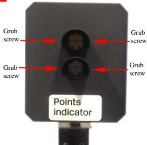
Remove two M8x10 grub screws from each visor using an M4 Allen key
