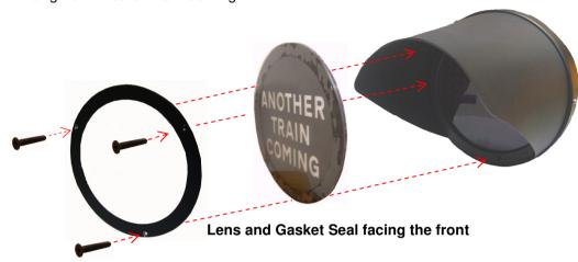
Note: Tighten the three M4 x 35 Stainless Steel C'Sunk Pozi Head Screws at 1.2NM Torque.
