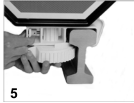
5 Pull release catch to remove.
