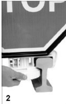
2 Twist cam to lock.
