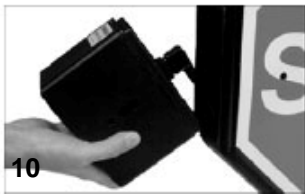
10 Withdraw battery box.
