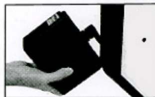
10 Withdraw battery box.
