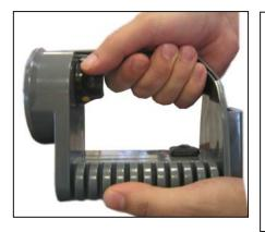
The Railway LED Handlamp is a 3 aspect device comprising of Red, Green and White colour output. Rotate the switch as shown to select the desired colour aspect indicated on the switch knob. The colour can be viewed from the top of the lamp (see **Fig.1**) through the colour indicator lens. The switch has eight positions - four 'ON' and four 'OFF'.
