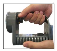
The Railway LED Handlamp is a 4 aspect device comprising of Red, Yellow, Green and White colour output. Rotate the switch as shown to select the desired colour aspect indicated on the switch knob. The colour can be viewed from the top of the lamp (see Fig.1) through the colour indicator lens. The switch has eight positions - four 'ON' and four 'OFF'.
