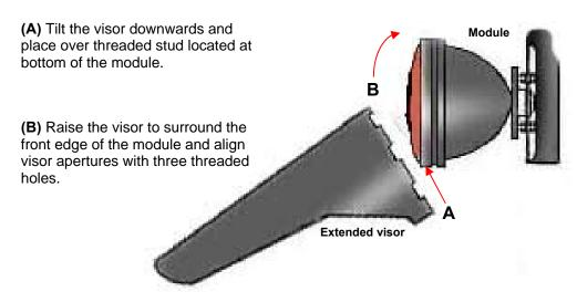
**(C)** Secure visor with M4 plain washer, M4 spring washer and M4x12 long button socket head screw s/s using 2.5mm Allen key <u>provided</u>.
