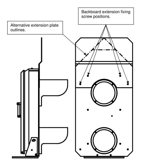
Signal with upper backboard extension fitted. (Full upper backboard extension shown)
