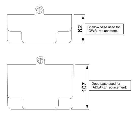
The correct base should be selected to suit the particular signal requirements.
