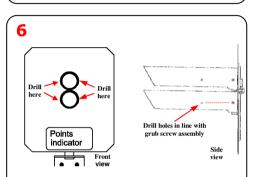
Using the pre drilled holes as a guide, drill a 5.2mm hole to each side through both existing visors
