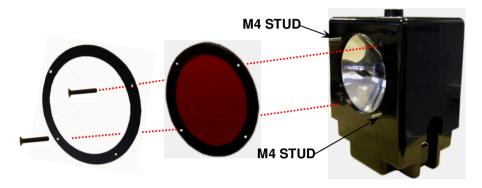
Position Filter / Gasket & Lens Clamp onto the M4 STUD, 35 LG and tighten
