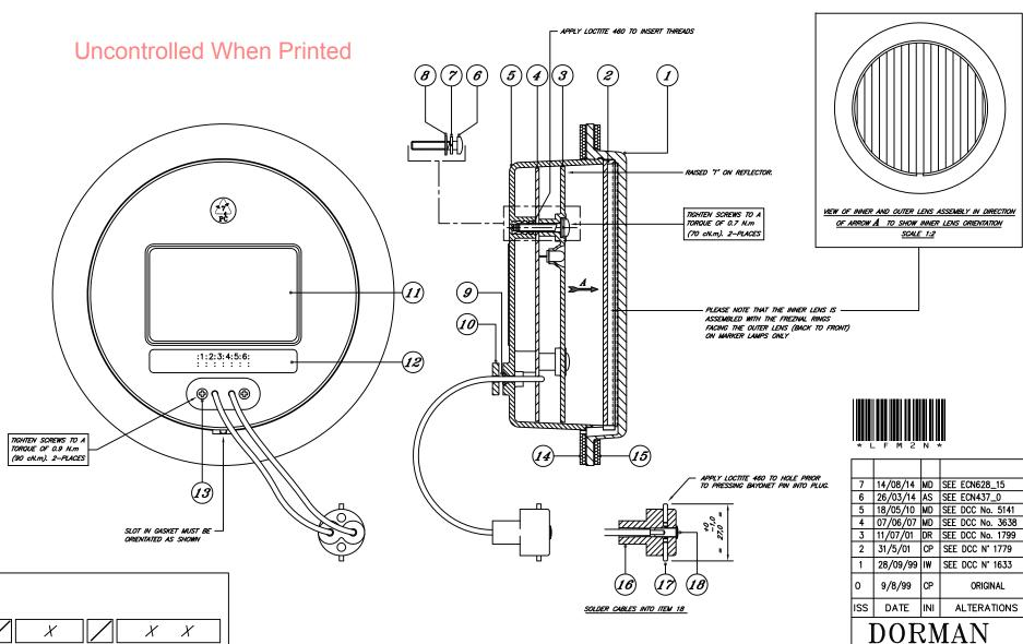
NOTE - MARKER LAMP WITH FLANGE DIA 'A' (162 MM) SHOWN
