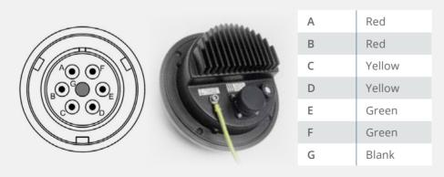
\*Contact G is unused and will be fitted with a blanking plug
