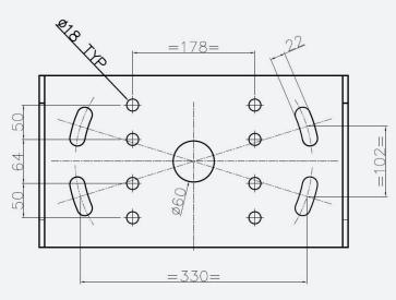
Baseplate designed to be used on either BRS-SM-2076 or BRS-SM-65/10 Mountings.
