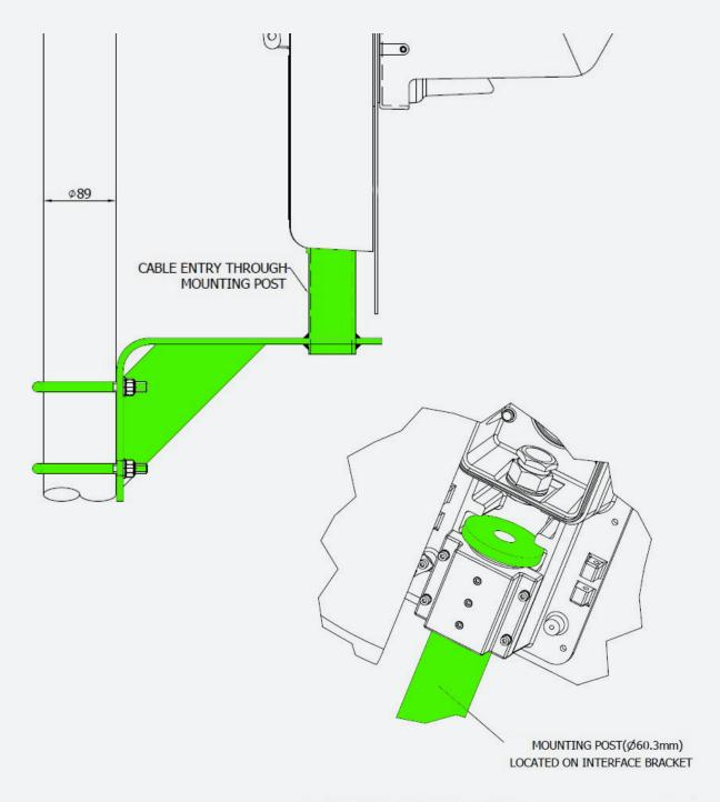
DETAIL OF POST MOUNT & CLAMPING ARRANGEMENT.
