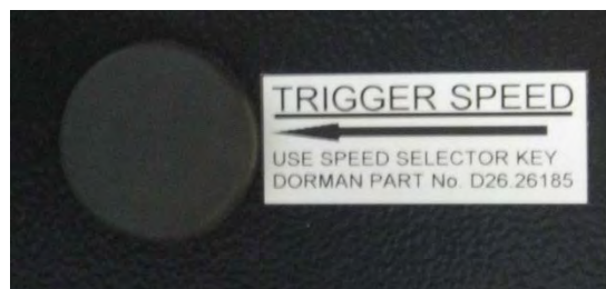
Bung fitted correctly after adjustment
